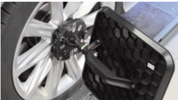
Practical magnetic clamps ensure high set-up speed
